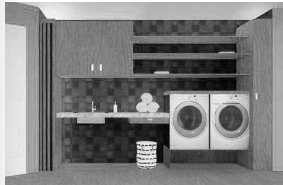
Laundry with roll under sink, elevated appliances, and pull out storage and drying racks
